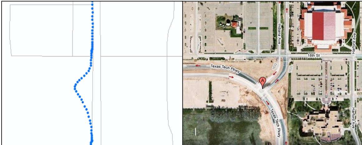
Figure 6 Possible Missed Trip End Revealed as New Intersection with Google Satellite Imagery.
