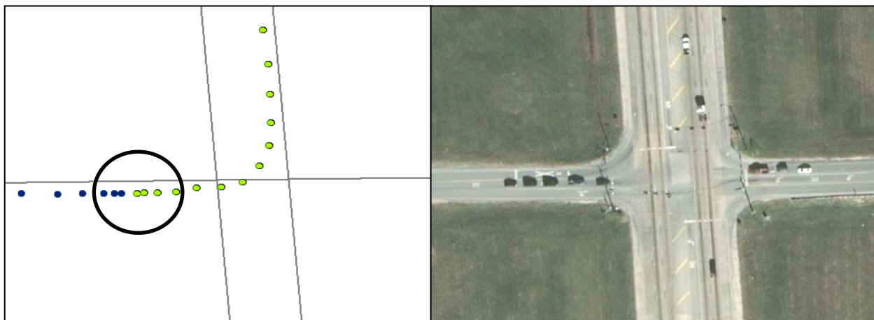
Figure 3 Invalid Trip End Identified in a GIS and Verified Using Google Maps Satellite Imagery.
