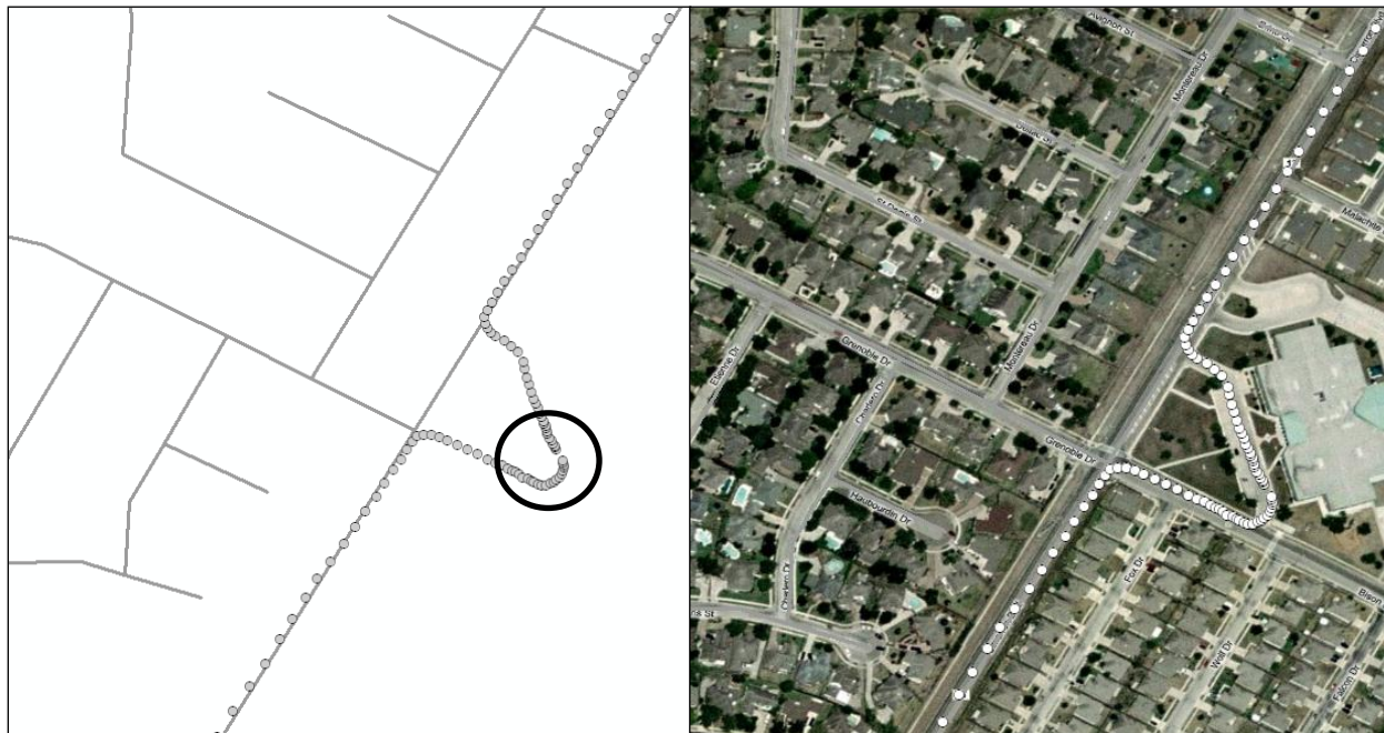
Figure 7 Missed Trip End and Outdated Road Network Shown in ArcGIS with Bing Aerial Imagery.
